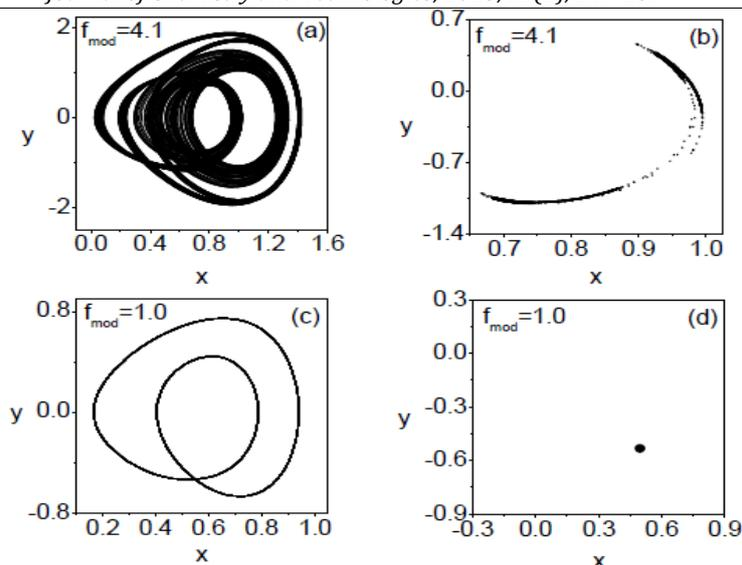
Fig. 6. Phase portraits and the corresponding Poincaré maps for the system (Eq.8) driven by a periodic modulus of sine wave force for two values of  $f$  chosen in the chaotic and periodic regions in Fig.5(c). The values of the other parameters of the system fixed as  $\alpha = -1$ ,  $\beta = 5.0$ ,  $\mu = 0.4$ ,  $\Gamma = 0.5$  and  $\omega = 1.0$
