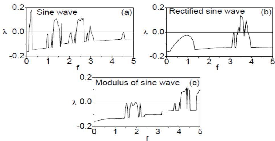
**Fig. 1. Lyapunov exponents  $\lambda$  versus the parameter  $f$  for the system (Eq.8) driven by a (a) sine wave (b) rectified sine and (c) modulus of sine wave forces. The values of the other parameters of the system fixed as  $\alpha = -1$ ,  $\beta = 5.0$ ,  $\mu = 0.4$ ,  $\Gamma = 0$  and  $\omega = 1.0$ .**
