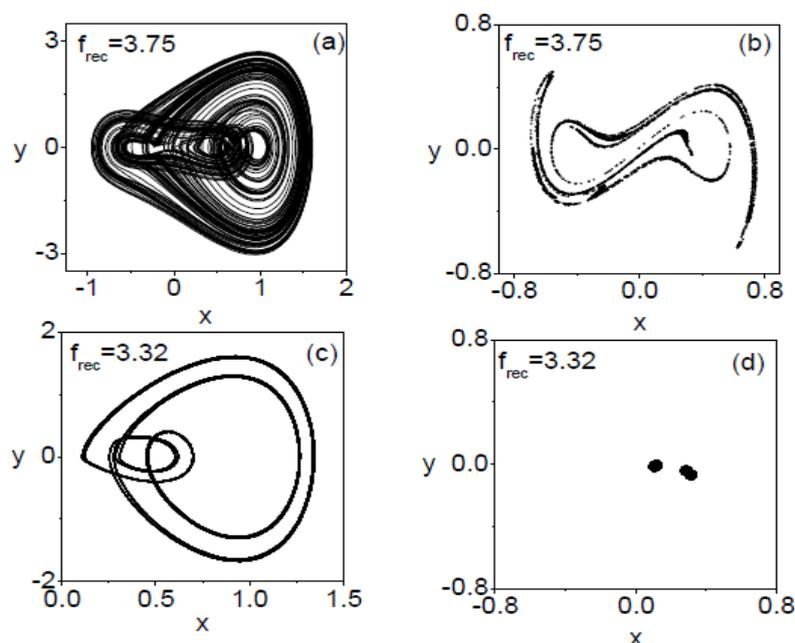
Fig. 9. Phase portraits and the corresponding Poincaré maps for the system (Eq.8) driven by a periodic rectified sine wave force for two values of  $f$  chosen in the chaotic and periodic regions in Fig.8(b). The values of the other parameters of the system fixed as  $\alpha = -1$ ,  $\beta = 5.0$ ,  $\mu = 0.4$ ,  $\Gamma = 0.25$  and  $\omega = 1.0$
