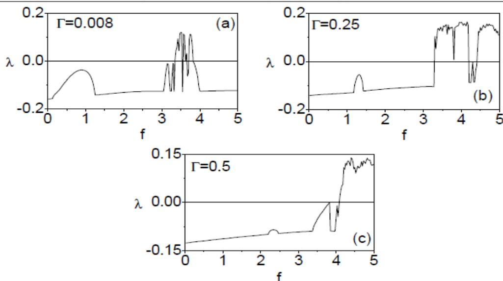
Fig. 8. Lyapunov exponents  $\lambda$  versus the parameter  $f$  for the system (Eq.8) driven by a periodic rectified sine wave force for three values of  $\Gamma$ . The values of the other parameters of the system fixed as  $\alpha = -1$ ,  $\beta = 5.0$ ,  $\mu = 0.4$  and  $\omega = 1.0$
