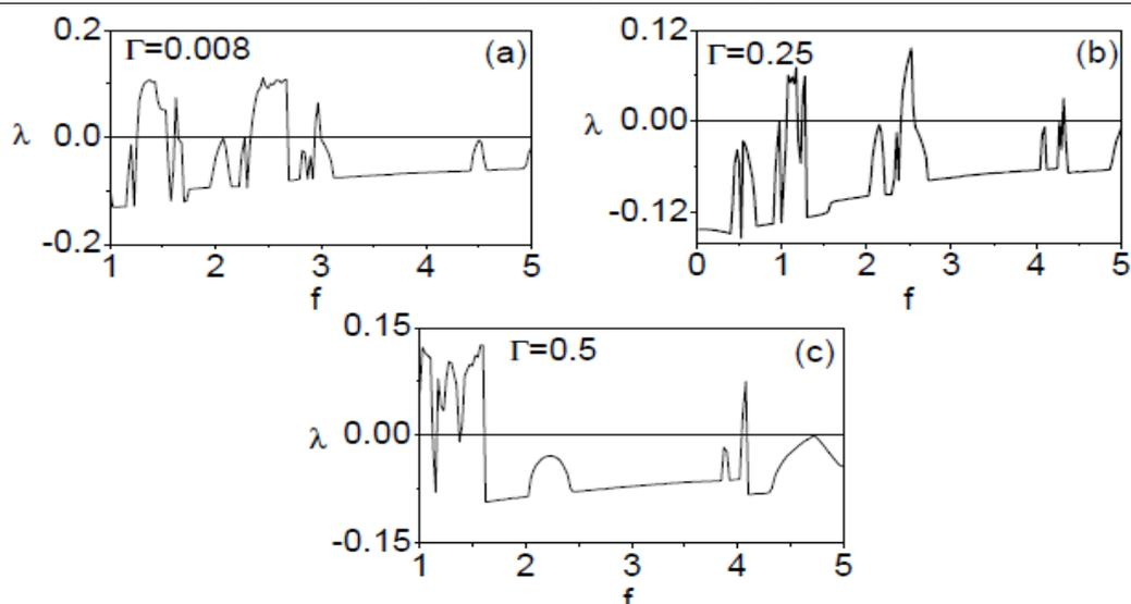
Fig. 2. Lyapunov exponents  $\lambda$  versus the parameter  $f$  for the system (Eq.8) driven by a periodic sine wave force for three values of  $\Gamma$ . The values of the other parameters of the system fixed as  $\alpha = -1$ ,  $\beta = 5.0$ ,  $\mu = 0.4$  and  $\omega = 1.0$
