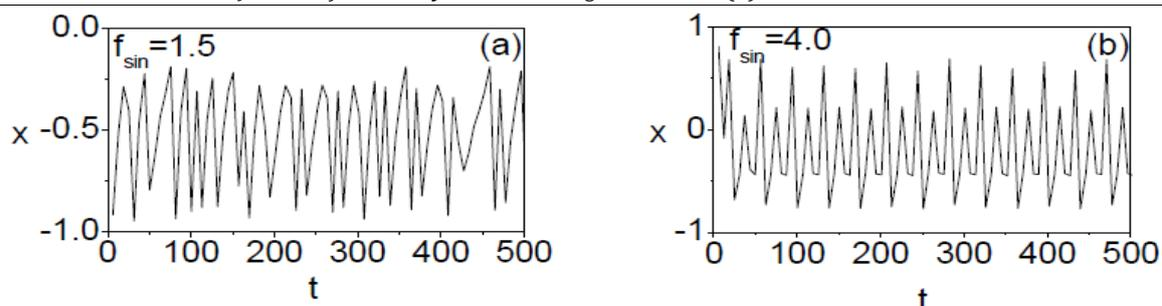
Fig. 4. Time evolution of the system (Eq.8) is driven by a periodic sine wave force for two values of  $f$  chosen in the chaotic and periodic regions in Fig.2(c). The values of the other parameters of the system fixed as  $\alpha = -1$ ,  $\beta = 5.0$ ,  $\mu = 0.4$ ,  $\Gamma = 0.5$  and  $\omega = 1.0$ .
