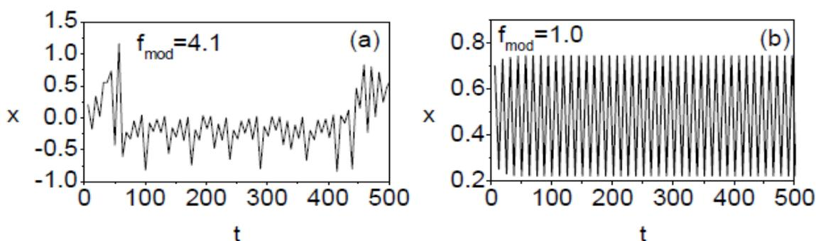
Fig. 7. Time evolution of the system (Eq.8) driven by a periodic modulus of sine wave force for two values of  $f$  chosen in the chaotic and periodic regions in Fig.5(c). The values of the other parameters of the system fixed as  $\alpha = -1$ ,  $\beta = 5.0$ ,  $\mu = 0.4$ ,  $\Gamma = 0.5$  and  $\omega = 1.0$ .
