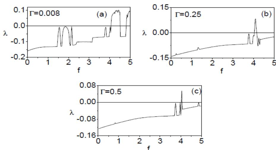
Fig. 5. Lyapunov exponents  $\lambda$  versus the parameter  $f$  for the system (Eq.8) driven by a periodic modulus of sine wave force for three values of  $\Gamma$ . The values of the other parameters of the system fixed as  $\alpha = -1$ ,  $\beta = 5.0$ ,  $\mu = 0.4$  and  $\omega = 1.0$
