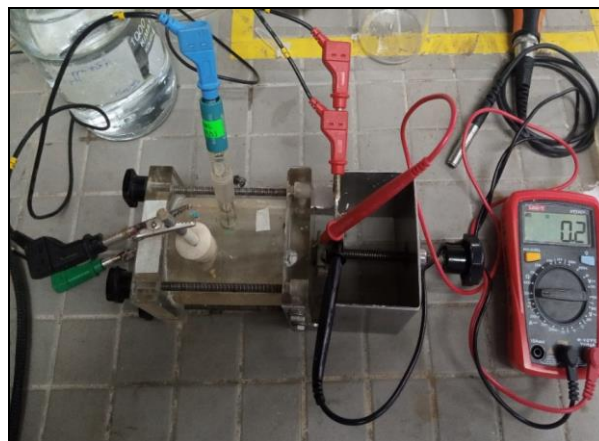
Fig. 3. The coated blocks were connected to the working electrode (red colored plug), a stainless-steel rod was inserted as the reference electrode (black colored plug), and the same counter electrode was used in each EIS test (blue colored plug).
