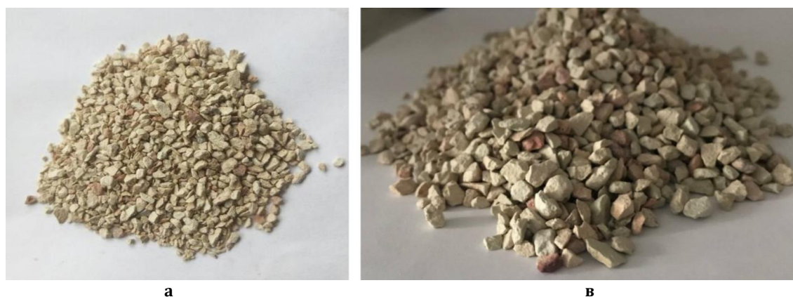
Fig. 1. Natural sorbent of the Sokyrnytskyi deposit with a fraction of 2.5–5.0 mm: A – native zeolite, B – spent zeolite
