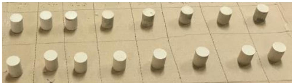
Fig. 2. Phosphate pellets obtained under the following pressures: 80, 100, 140, 200, 240, 300 and 340 bars
