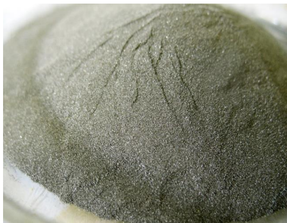
Fig. 7 Tungsten powder obtained by the W-Ni-Fe alloy leaching
