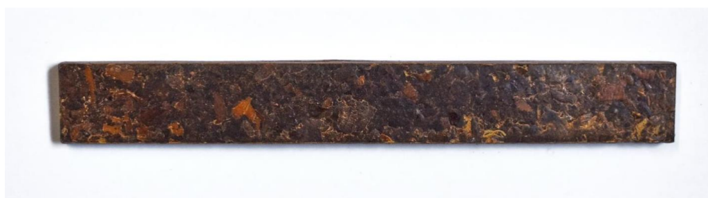
Fig. 3. A briquetted sample of solid fuel obtained from the acorns of the common oak ( Quercus robur ).
