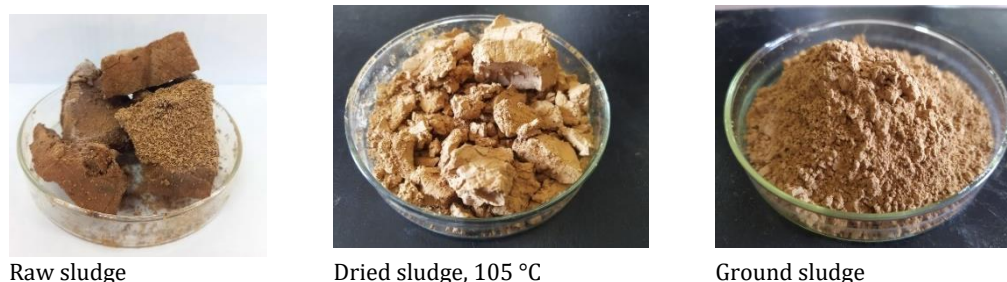
Fig. 1. WTS before modification
