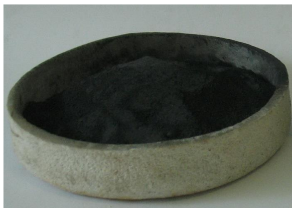
Fig. 8 Tungsten carbide powder obtained as a result of leaching of WC-Ni
