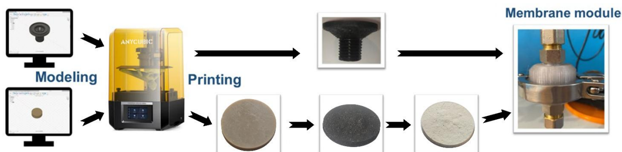
Fig. 9. Schematic illustration of using DLP technology to create ceramic membrane modules
