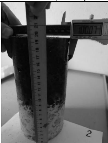
Fig. 2. Image of concrete sample No. 2 (degree of oil saturated – 56%)
