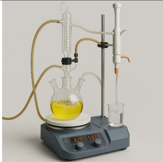
Fig. 3. Experimental setup used during the third stage of the synthesis process: a three-necked flask equipped with a magnetic stirrer, thermometer, and reflux condenser
