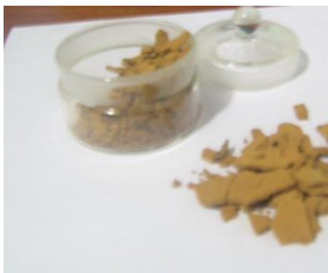
Fig. 2. The resulting iron-chromium catalyst before the grinding and tableting stage
