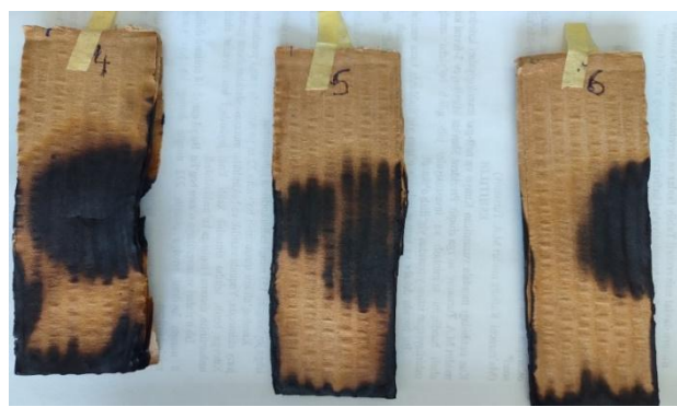
Fig. 12. Flame-retardancy test on cardboard samples
