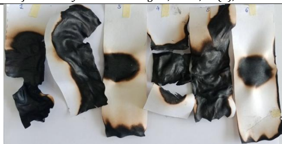
Fig. 11. Flame-retardancy test on paper samples
